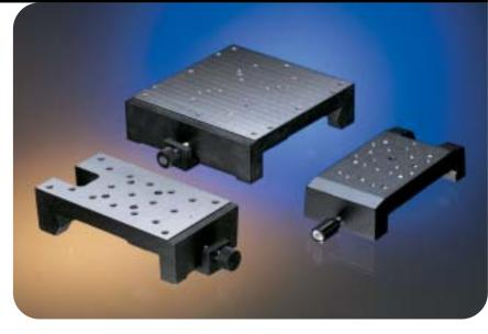
The Standard Carrier is an aluminum die-casting with machined rail contact faces. It clamps to the rail with a simple locking screw, and incorporates a vernier which allows the bench scale to be read to 0.1 mm. The Standard Carrier is ideal for use with the Aluminum Low Profile Rail and accepts Posts and Slides from the Triangular Rail range.
